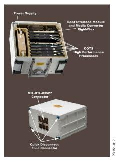
The CEEU is contained within a standard 11 MCU liquid-cooled chassis.
