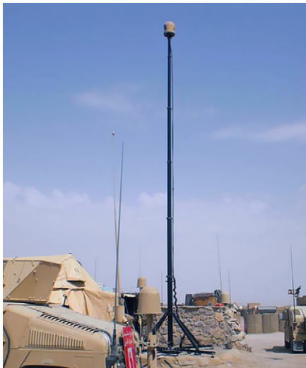
Integrated base reduces footprint without guy wires in rugged deployment locations.
