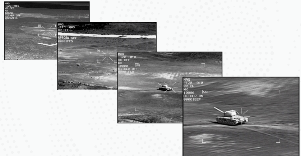
Infrared images with enhanced image processing show increasing levels of magnification from wide field-of-view to very narrow field-of-view.
