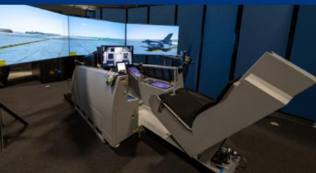
The Weapons Tactics Trainer is a modified cockpit and visual system that allows weapons and tactical training. It can be used as a standalone training device or be fully integrated with other devices as a force multiplier.
