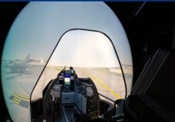
The Full Mission Trainer is a fully immersive, networked, high-fidelity, visual, aural, and tactile simulation of the F-16 aircraft cockpit with multi-ship network capability that enables pilots to train like they fly.
