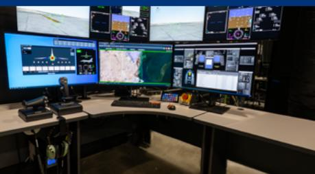
The Instructor Operation Station (IOS) offers a full suite of controls and views for the instructor/operator to perform scenario planning, training execution and real-time monitoring.
