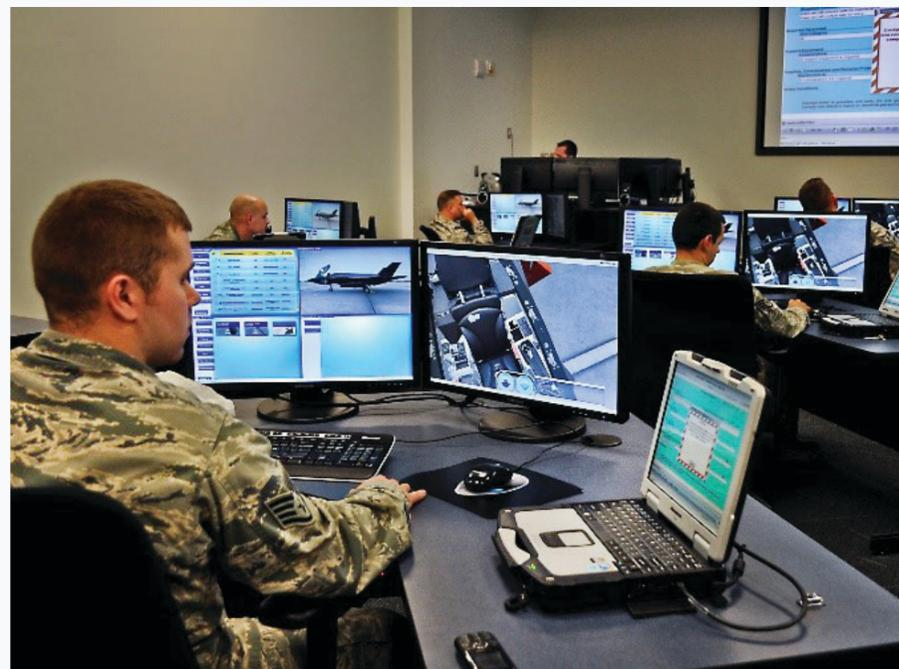
and proper use of the ALIS portable maintenance aid. Instructors are provided a dedicated operating interface enabling capabilities including lesson assignments, student progress monitoring, automatic grading, intercoms, and video switching. The instructor operating station controls and supports up to 12 student stations. While the ASMT has trained thousands of maintainers in F-35 training centers, the system can be utilized at the squadron level for refresher training.
