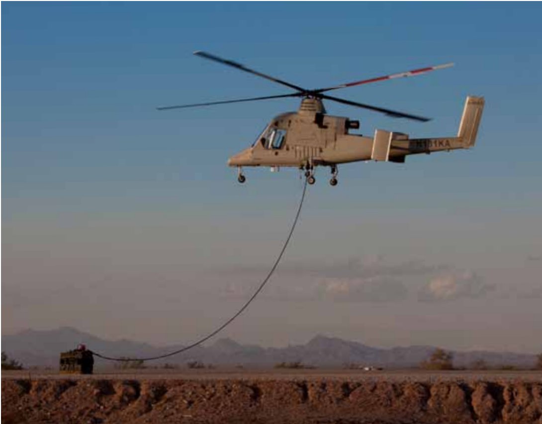
A K-MAX UAS lifts 1,500 pounds during contractor flight tests at Yuma Proving Ground, AZ, in January 2010.
