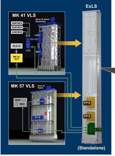
The lightweight mechanical launcher structure facilitates drop-in/snap-in capability by having the same mechanical interfaces as the existing VLS canisters. The launcher features Open System Architecture and Open Software and Cell Based Electronics.
