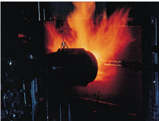
2000°F flame test for 15 minutes.
