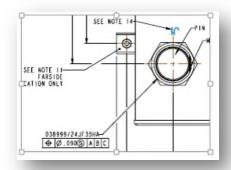
Example: MIL-DTL-38999 has the requirements for the hole size for the connector illustrated as well as torque requirements.
