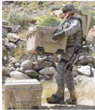
Allows One Soldier to Lift Loads, Maintains Normal Lifting Range of Motion and Keeps the Center of Gravity Close to the Soldier
