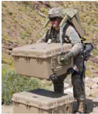
Allows One Soldier to Lift Loads, Maintains Normal Lifting Range of Motion and Keeps the Center of Gravity Close to the Soldier
